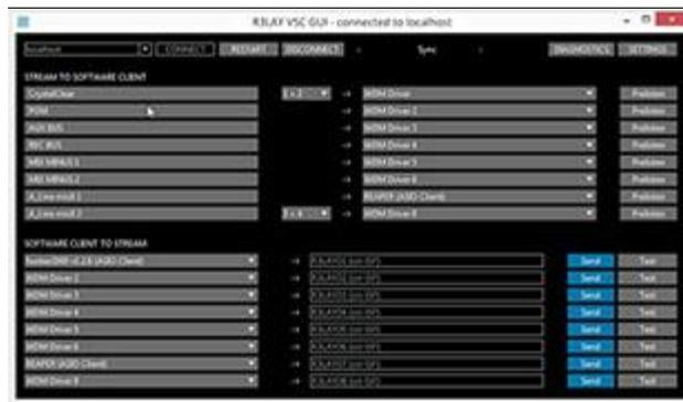
To be able to communicate all 16 channels with a PC you need a software driver such as the LAW0 RELAY Matrix shown above. The AES67/USB card of the AXUM system can communicate with all equipment which is AES67 compliant. When speaking about Dante there are two flavors : - Native Dante equipment (This is older equipment which does ONLY support native Dante and is NOT AES67 compliant) - Dante +
